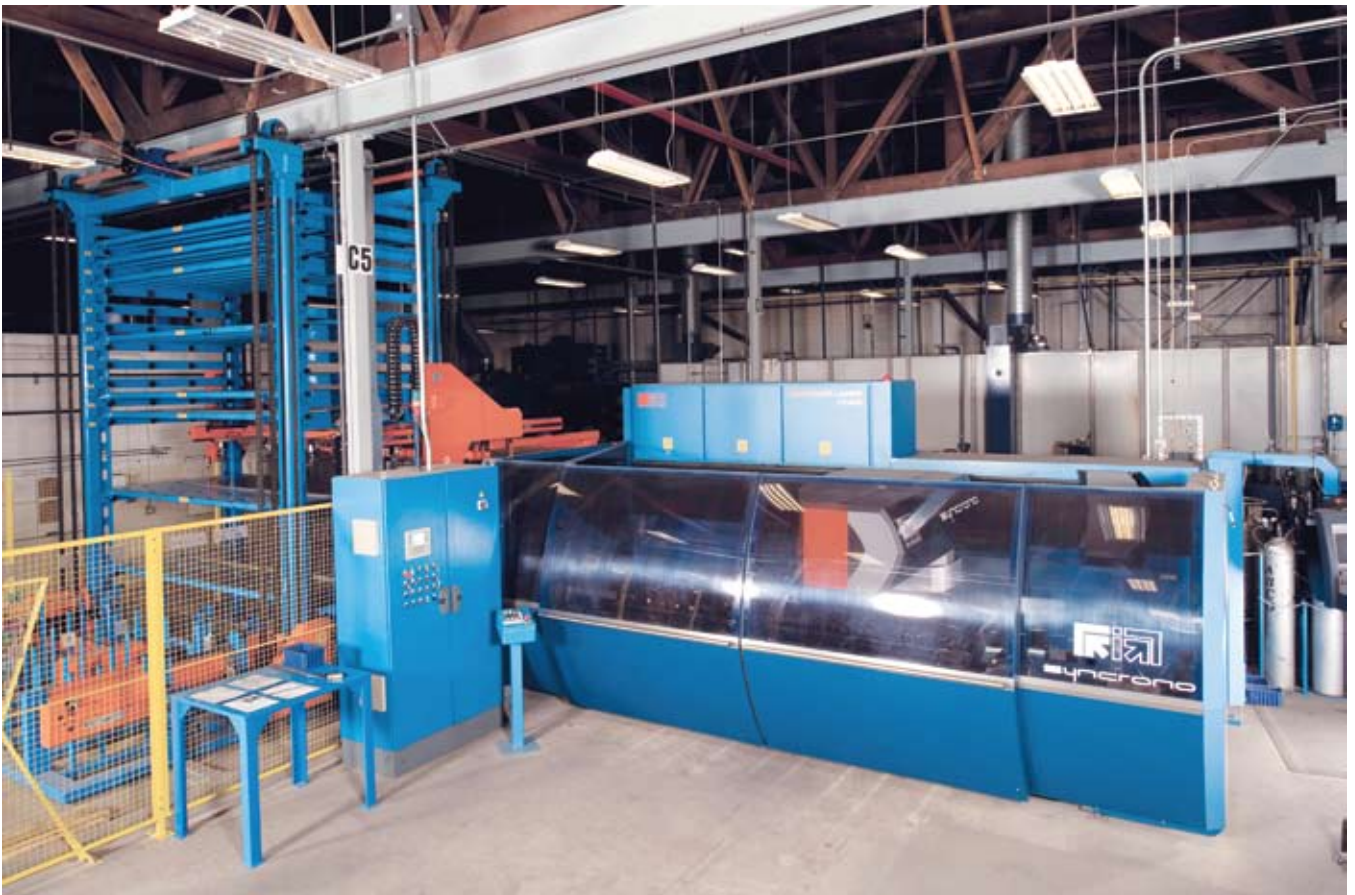
The Prima Sincrono laser with the TowerServer in the background. The system is capable of Lights Out operation, a feature that appealed to Rob Marelli.
