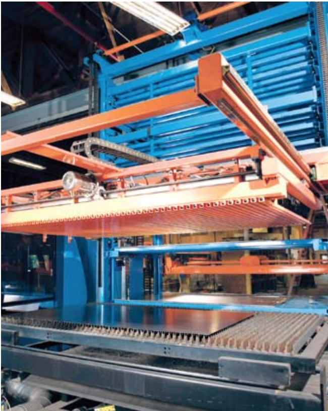
The Prima Sincrono laser with the TowerServer in the background. The system is capable of Lights Out operation, a feature that appealed to Rob Marelli.
