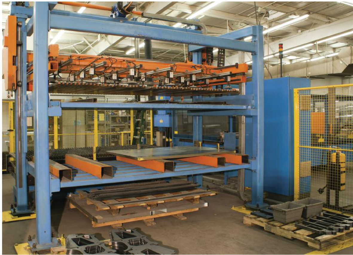
In 2006, Pulverman purchased a second Platino laser with a load/unload. According to Yermal, the flexibility of the load/unload gives Pulverman the ease of loading and unloading sheets, just like on the large tower. All the operator needs to do is touch a few buttons to unload a scrap sheet and load a new sheet. With the load/unload, the company can just load the material that it is running at that moment.
