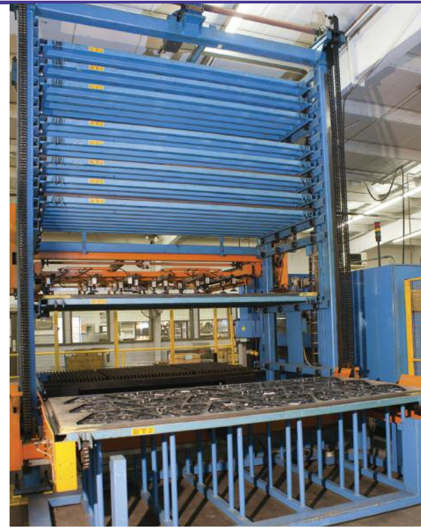
Prima’s 10-shelf TowerServer allows easy loading/unloading for blanks and processed sheets. It has an elevator for loading and unloading the pallets on and off the tower, and features single sheet separating, control systems, and sheet reference.
