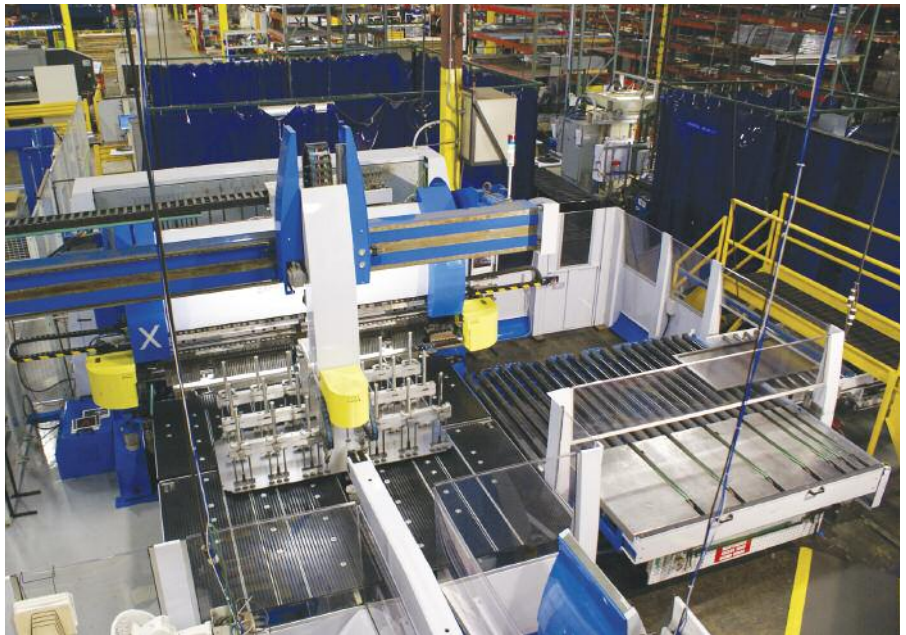
Finn-Power worked with Emerson on designing a conveyor from the EBe to the next operation, welding. The company wanted to do one-piece flow because the majority of its parts get welded with either a TIG or a spot welding process. Finn-Power modified the logic in the PLC and modified the unloader rails so the parts have two ways to exit: Directly out of the machine down a conveyor to the welder or they can exit at a 90 degree angle for unloading.
