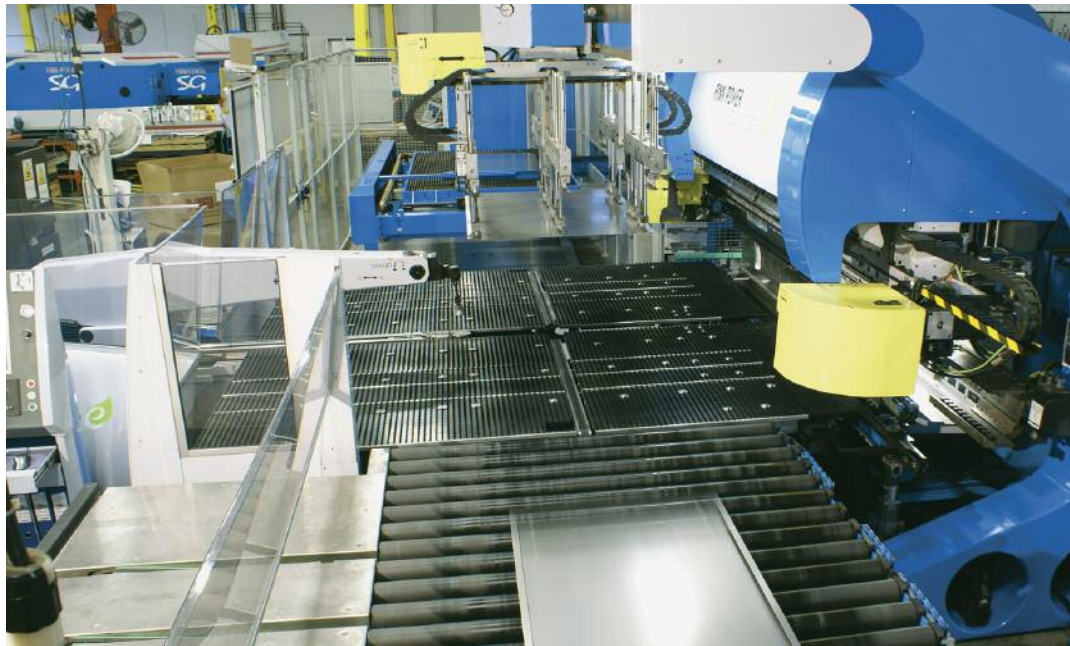
The EBe servo electric Express Bender is a bending solution that is designed specifically for each fabricator's production requirements to achieve maximum productivity, quality, and repeatability. The bending operation is fully automated, from the loading of flat punched parts to unloading of the finished product.
