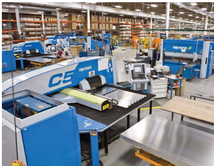
Figure 3 A Finn-Power C5 turret punch press and a servo-electric E series press brake were the first pieces of metal fabricating equipment Orion purchased when it moved its fabrication activities in-house in 2004.
