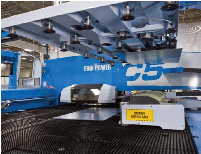
Figure 4 The acquisition of the C5 Compact Express with automated material loading and unloading in 2006 addressed workers' fatigue associated with moving the large sheet metal blanks.
