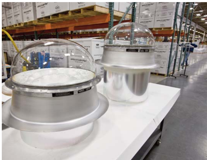
Figure 2 The Apollo® Light Pipe captures sunlight through its dome, feeds the light through a sealed "light pipe," and focuses it into a building, eliminating the need for electrically generated light for part of a day.
