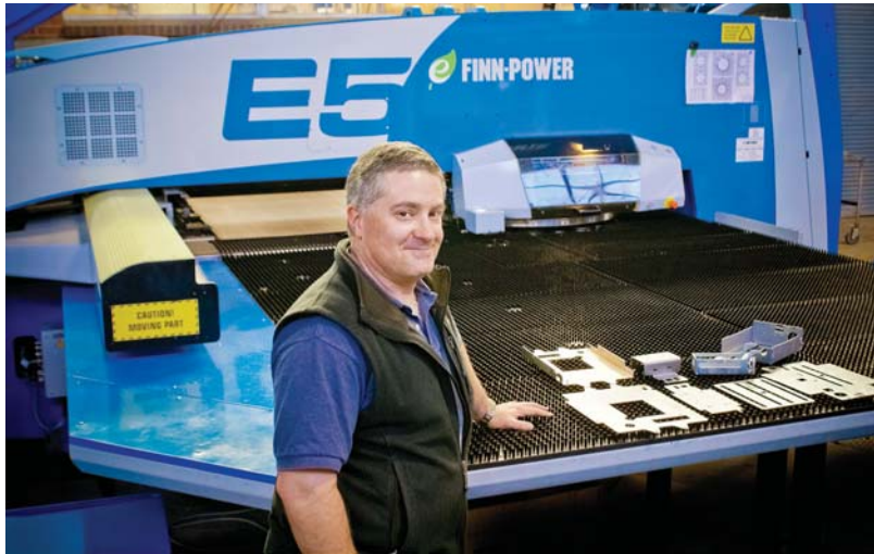
Tim Morroni's company, Electric Equipment & Engineering Co., utilizes the Finn-Power E5 Compact Express to produce power distribution and transfer systems in all shapes and sizes from 200 – 4,000 amps.
