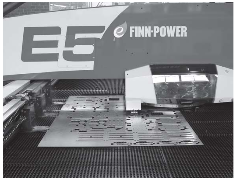
The tapping feature of the E5 has also paid a large dividend to EEE. The company chose a six-station, servo-driven tapping unit.
