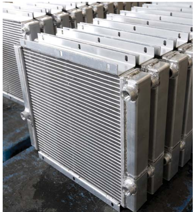
Radiator components manufactured on the Finn-Power Shear Genius System.
