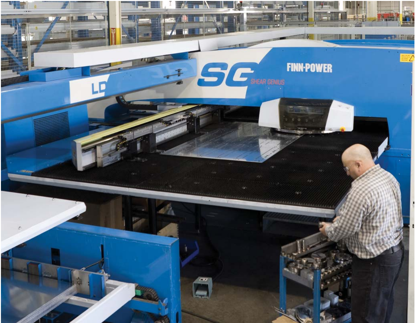
The Shear Genius cell with loader in front, turret punch press, Night Train Material Management System. Man in front is inspecting tooling.
